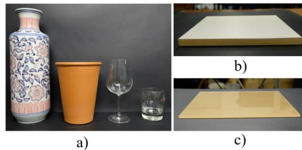
Figure 2: Specimens and substrates used to test the adhesives: a) ceramic vase, terracotta pot, wine glass, flat glass, b) acrylic substrate, and c) painted MDF substrate.
