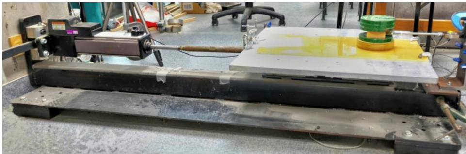
Figure 7: Unidirectional friction test setup to determine static and dynamic friction of coefficients.
