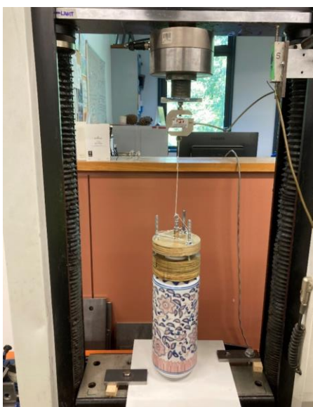
Figure 3: Direct tension test to determine adhesives' tensile properties.
