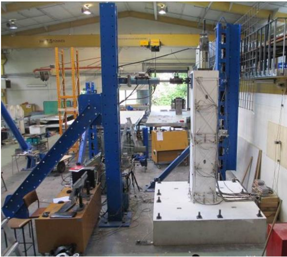
(a) Typical column test setup under uniaxial loading
