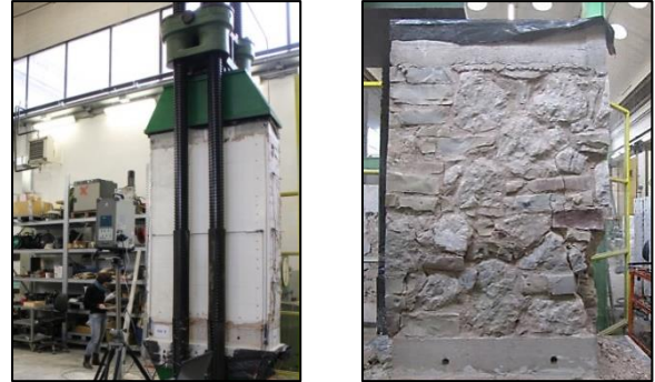
Figure 6: Compression test and failure mode [30]
