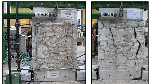
Figure 7: Shear-compression test and failure mode [30].
