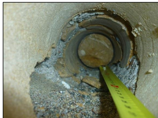
Figure 3: Execution of boroscopy test [www.expin.it].
