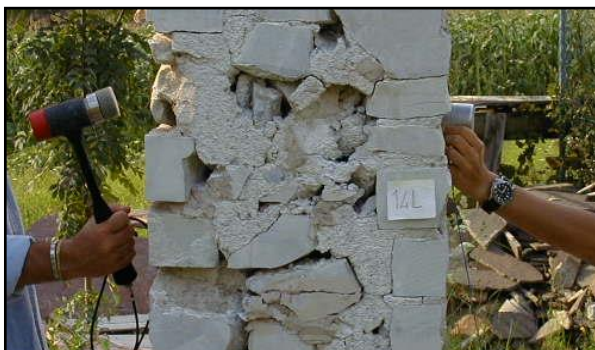
Figure 2: Example of direct sonic pulse velocity test [Source: University of Padova].
