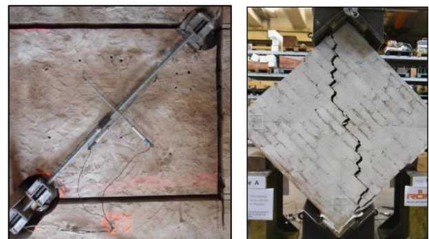
Figure 8: In-situ and laboratory diagonal compressive test undertaken using two different set-up configurations [Source: University of Padova].
