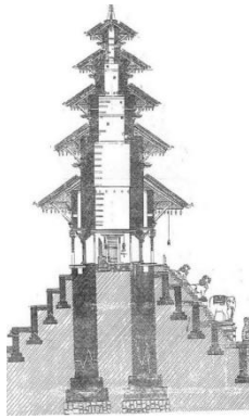
(b) Cross-section showing foundation and wall thicknesses [35]
