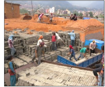
(d) Stacking of 'raw' bricks in the kiln and isolation cover
