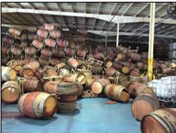
(b) Collapse of two barrel racks [64]
