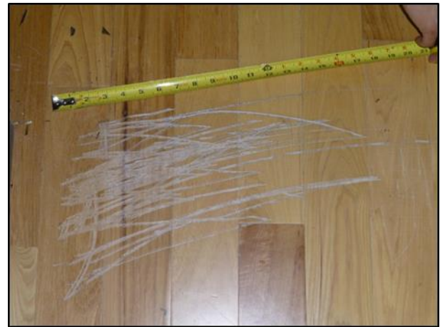
(a) Scratch marks due to cabinet motion
