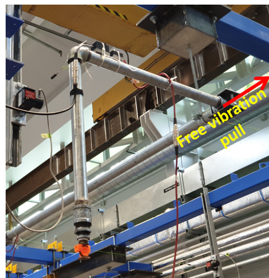
Figure A10: Location of free vibration pull for snap-back test.
