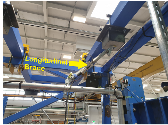
Figure A8: Longitudinal brace on branch pipe.
