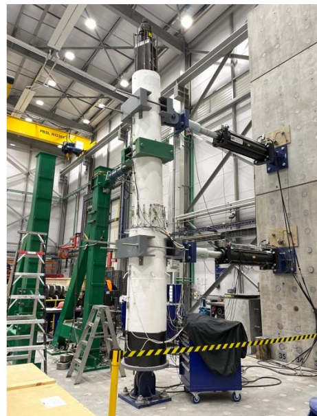
Figure 4: Schematic illustration and photographic image of the test setup for 1/3-scaled bridge pier with DCR connection.
