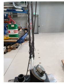
(b) Damage around the bracket.
