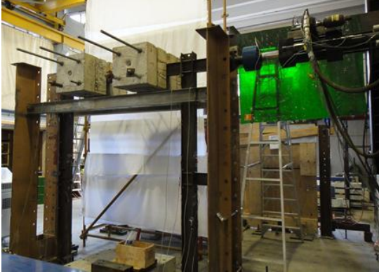
Figure 14: Steel moment resisting frame specimen (MRF) used in the experimental validations.
