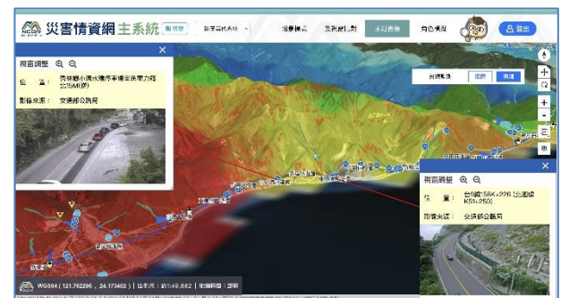
Figure 17: Real-time monitoring rainfall impact on the transport routes north of Hualien City (critically vulnerable spots on Highway 9 that had been cut off several times by the earthquakes, rockfalls and debris flows following heavy rain). Colours indicated the amount of rainfall in the areas.
