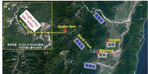
Figure 28: Impact assessment of a quake dam on upper stream of Wanli Creek (identified on 3 April 2024 following the M_w 7.4 mainshock) [24]. The dam was approximately 20km from the downstream Wanrong Village that lies 10m above the riverbed.
