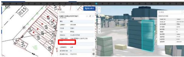
c) Left image shows the rapid building assessment results following the Hualien Earthquake, with red box highlighting the building (shown in the right image) receiving a red placard.
