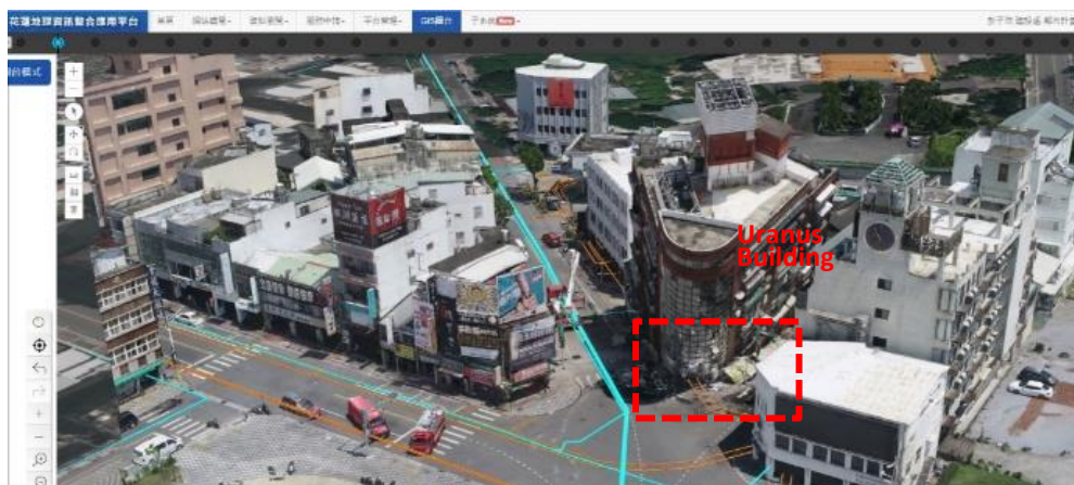
Figure 20: 3D spatial relationship between the collapsed Uranus Building and underground lifelines (electricity – orange lines, water – blue lines) following the M_w 7.4 earthquake on 3 April 2024. Power and water supplies to the neighbouring properties were compromised for over two weeks until the demolition of the Uranus Building was completed. Red box indicates the lifelines (electricity) underneath the collapsed building.
