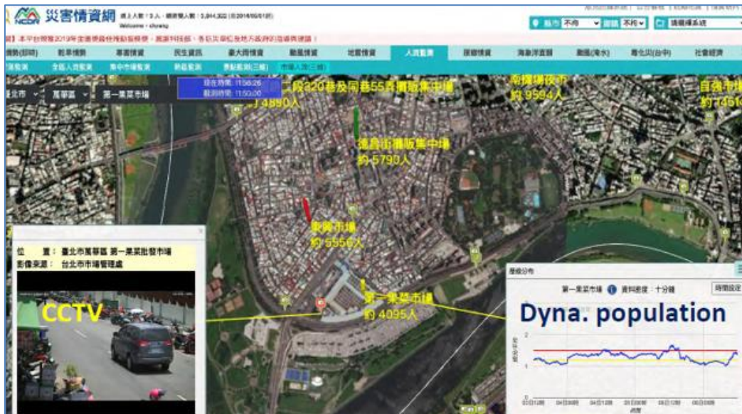
Figure 6: PRISM monitoring crowd status around markets in Taipei City during COVID through analysing telecommunications flow data (every ten minutes, right insert) and CCTV footage (left insert).
