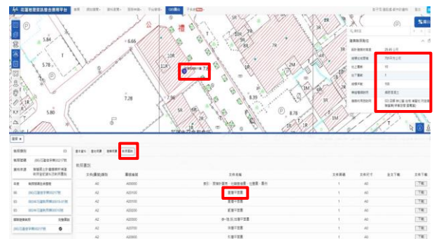
Figure 19: Retrieving records for a multi-storey building that collapsed on 23 April 2024 following two aftershocks greater than magnitude 6. These records include full lifecycle of consent details, structural drawings and calculations, floor plans, and cadastral details.
