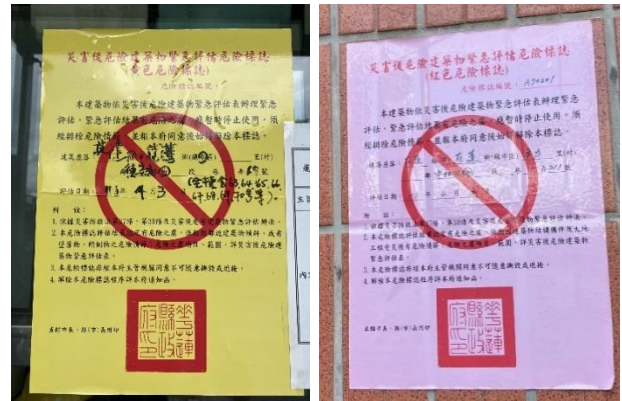
Figure 31: Examples of official post-earthquake building evaluation placards, showing yellow- and red-tag classifications.
