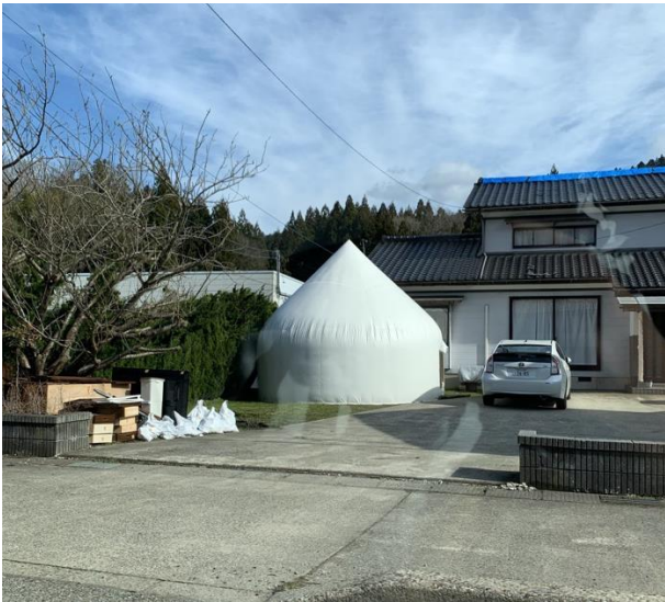
Figure 7: Thermally insulated emergency tents for red placarded homes, deployed from bulk storage in four locations around Japan.
