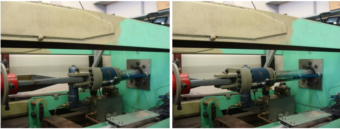
Figure 7: Maximum extension (left) and maximum compression (right) on first test cycle. Figure 8 shows that the forces just before and after the photograph at left was taken were substantially greater than those designed for.
