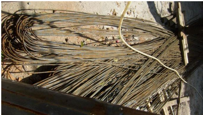
b) Plain reinforcing mild steel bars are commonly used.
