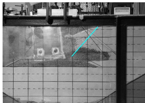
Figure 8: Displacement of caisson and deformation of backfill of test QW-01dry after shake3.
