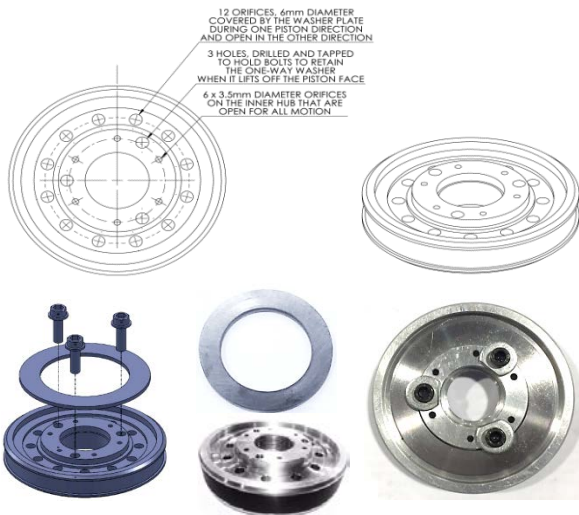
Figure 8: Scheme and photo of the modified piston.
