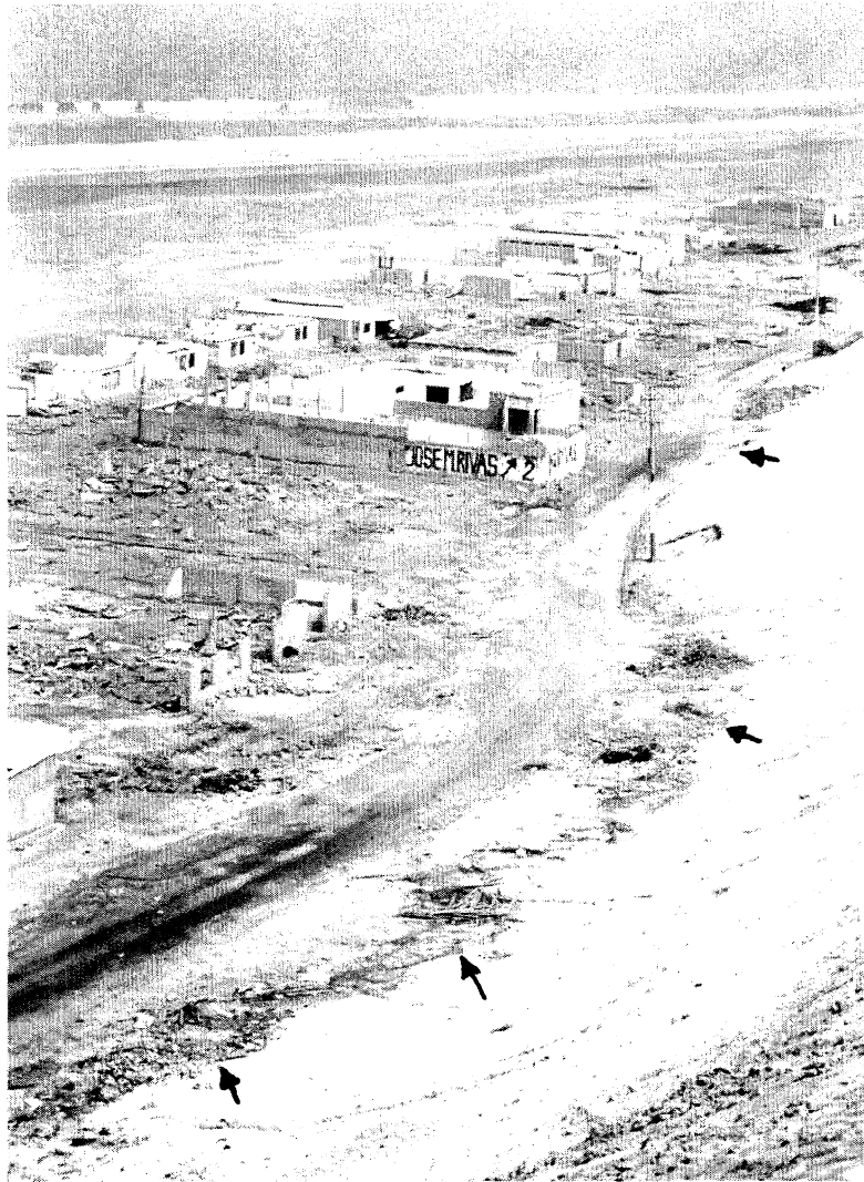
Figure 15. The settlement of Las Cuevas (southeastern continuation of Camana) as we saw it some five weeks after it was destroyed by the tsunami. Arrow points to a darkish line of water-washed debris at the base of the hill, which marks the maximum inland extent of the tsunami.
