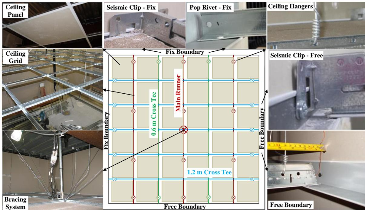
Figure 1: Typical layout and elements of an acoustical lay-in suspended ceiling system.
