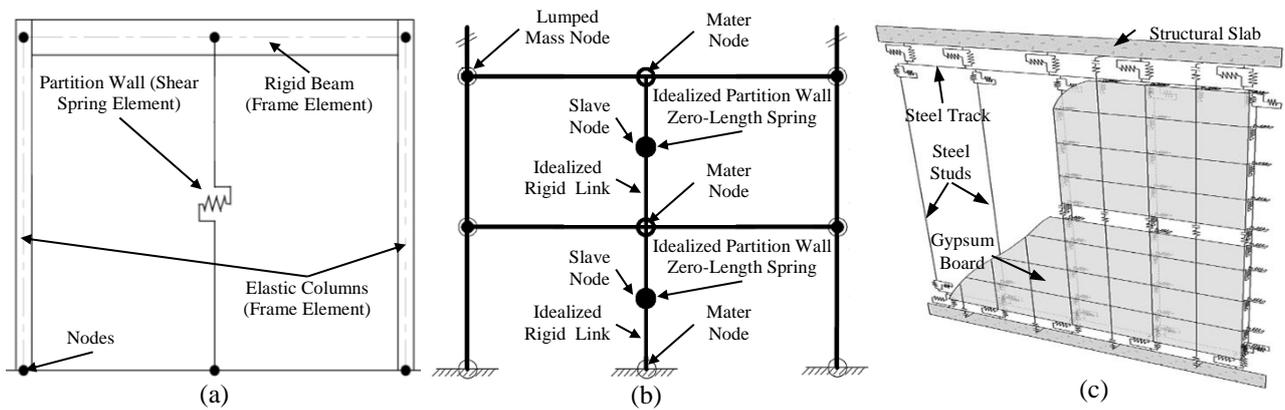
Figure 6: Examples of analytical studies on partition systems: (a) Davies *et al.* [40], (b) Wood *et al.* [94], (c) Rahmanishamsi *et al.* [95].
