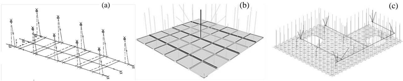
Figure 4: Typical layout and elements of a light-gauge steel-frame gypsum partition walls:(a) Yao [11], (b) Echevarria et al. [3], (c) Soroushian et al. [74].
