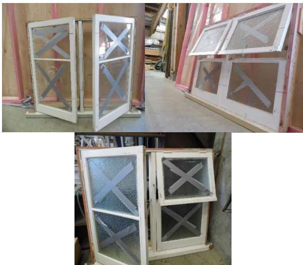
Figure 3: Wooden windows for residential fragility testing (Window 1 (Top Left): 1,290 mm wide x 1,030 mm high; Window 2 (Top Right): 1,320 mm wide x 990 mm high; Window 3 (Bottom): 1,325 mm wide x 1,050 mm high).
