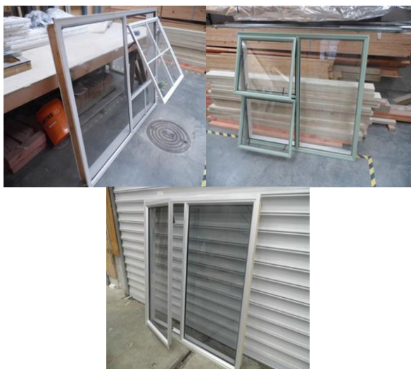
Figure 4: Aluminium windows for residential fragility testing (Window 1 (Top Left): 1,600 mm wide x 1,200 mm high; Window 2 (Top Right): 1,202 mm wide x 1,160 mm high; Window 3 (Bottom): 1,500 mm wide x 1,250 mm high).
