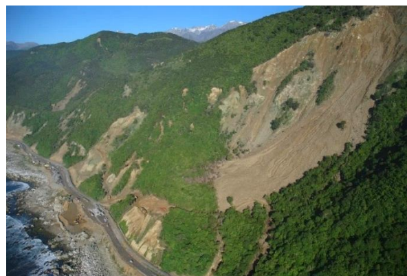
Figure 11: Examples of earthquake-damaged hillslopes in Half Moon Bay, north of Kaikōura, assessed as highly vulnerable to future failure in earthquake or rainfall events (see Figure 6 for location).
