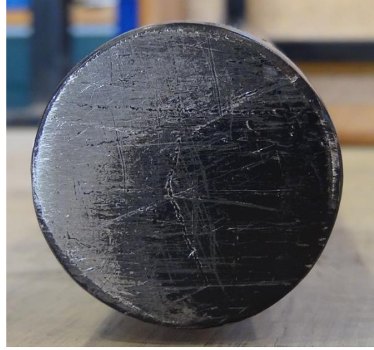
Figure 5: Uneven smoothness of the base of Desk 2 (similarly observed on all legs).
