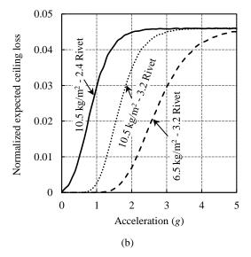
Figure 7: (a) Generalized expected loss curves of typical ceilings; (b) generalized and normalized (in terms of total building cost) expected loss curves of typical ceilings.
