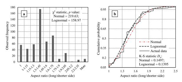
Figure 4: (a) Histogram of collected data; and (b) fitted cumulative distribution functions for ceiling aspect ratios.
