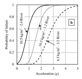
Figure 6: (a) Fragility curve for 12 m long suspended ceilings; (b) generalized fragility functions of typical suspended ceilings.
