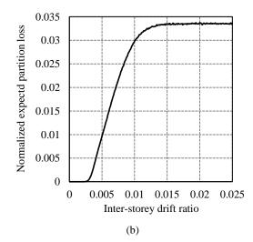
Figure 13: (a) Generalized expected loss for partitions; and (b) generalized and normalized (in terms of total building cost) expected loss curves for partitions.
