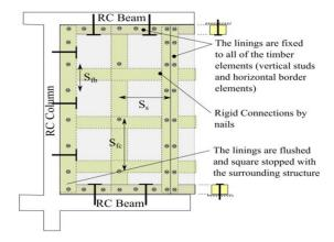
Figure 9: Typical timber-framed partition wall [35].
