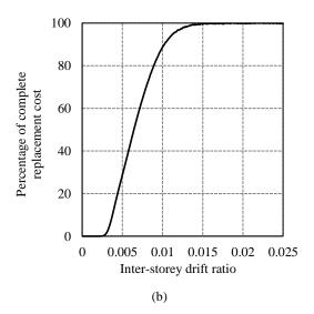
Figure 12: (a) Repair cost per partition area vs. inter-storey drift; and (b) percentage of complete partition repair/replacement cost.
