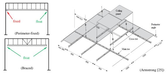
Figure 2: Schematic diagram and details of suspended ceiling.
