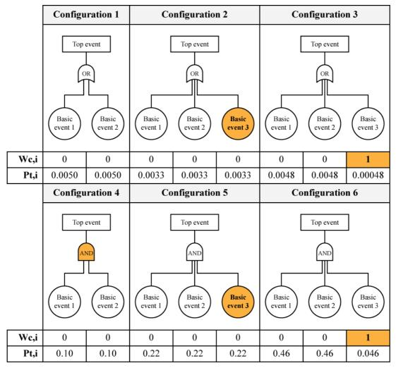
Figure 4: Performance objectives for each of the six fault tree configurations included in the parametric study. The selected resilience objective for the top event,  $P_{t,sys}$ , for all six configurations is 1% probability of failure in ground shaking with a particular return period.
