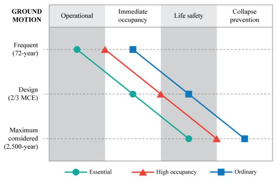
Figure 1: Seismic performance objectives for different building occupancies specified in the NEHRP Recommended Provisions (adapted from BSSC 2003 [11] and BSSC 2009 [9]).
