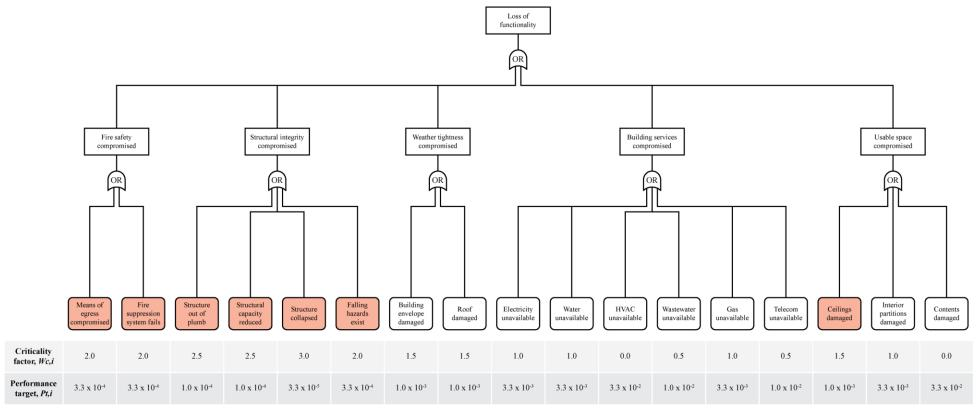
Figure 5: Fault tree for capturing loss of functionality in a generic commercial building, including criticality factors  $(W_{c,i})$  and performance targets  $(P_{t,i})$  for each "basic" event corresponding to a global resilience objective  $(P_{t,sys})$  of 10% probability of losing functionality in ground shaking with a particular return period.
