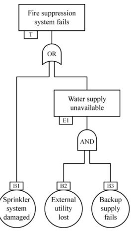
Figure 2: Example of a simple fault tree that captures failure of a hypothetical fire suppression system in a building.
