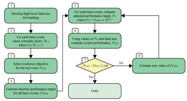
Figure 3: Methodology for computing risk-consistent performance targets for basic events from a global resilience objective for the top event in a fault tree.
