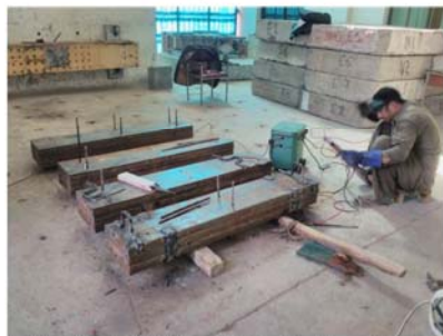
Stacking & Welding of Plates for Floor Blocks
