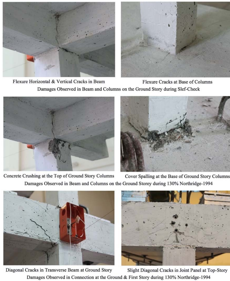
Figure 7: Damage observed in design conforming frame under significant test runs.
