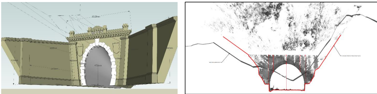
Figure 5: Left: 3D model from the laser scan of the Hataitai tunnel portals, used for architectural design. Right: Cross section at the portal of the upper tunnel of the Cable Car tunnels used for stability and structural analysis. The red line depicts ground topography captured from the laser scan, combined with topography from the Council Lidar data, depicted by the grey line.
