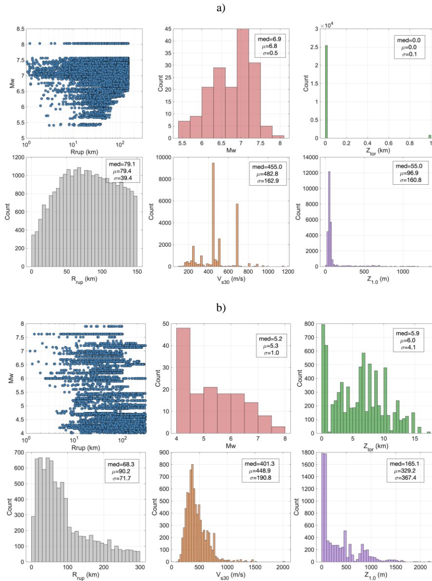
Figure 2: Distributions of the metadata in (a) the CyberShake NZ v20.11 database used in this study and (b) the subset of the NGA-W2 database used to develop BA18Corr .
