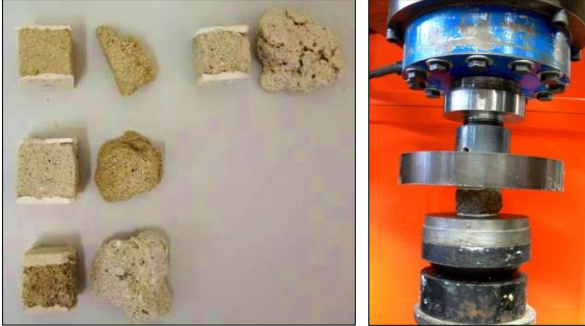
Figure 5: Irregular mortar samples (left) and mortar compression test (right).
