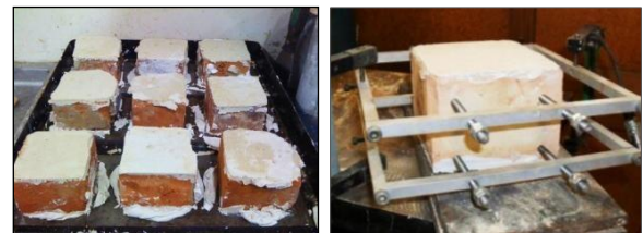
Figure 4: Gypsum plaster capping (left), and brick compression testing (right).
