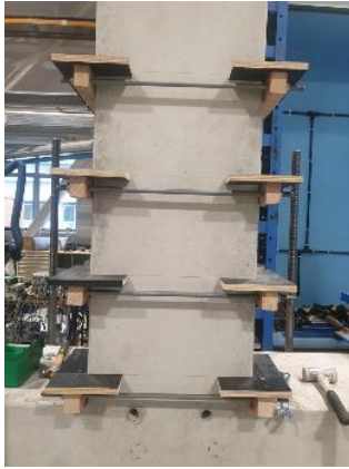
Figure 9: Supports made of wood to help installation of steel clamps.
