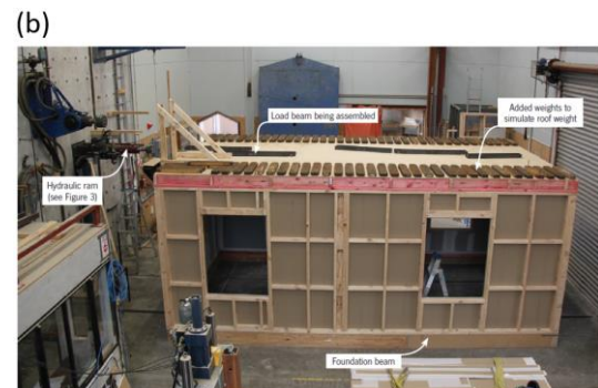
Figure 18: Test building [41]: (a) plan view; (b) test setup.
