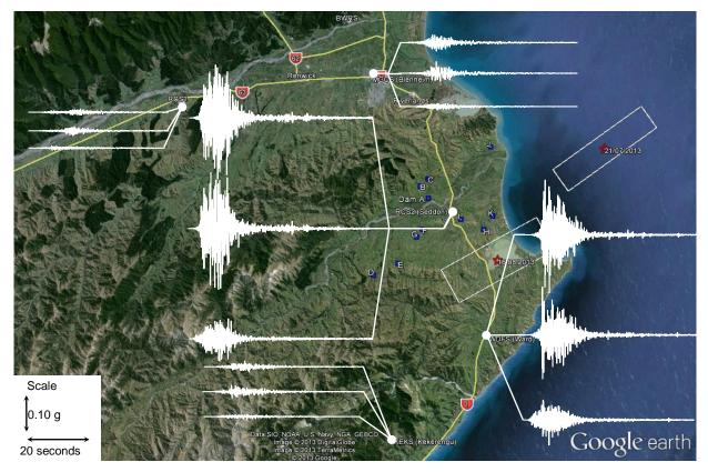
Figure 1: Ground motions observed in the Marlborough region from the 16 August 2013 M<sub>w</sub>6.6 Lake Grassmere earthquake. Fault normal (top), fault parallel (middle), and vertical (bottom) components are provided at each recording station. The inferred causative fault planes from the 16 August and 21 July earthquakes are also illustrated.
