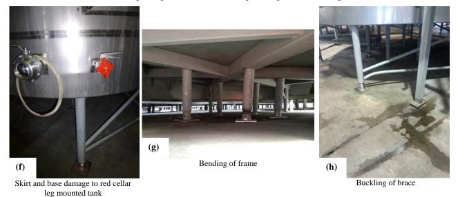
Figure 7: Various damage observations for leg mounted wine storage tanks.
