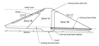
Figure 10: Typical embankment cross section.
