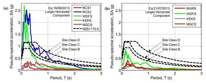
Figure 2: Larger horizontal response spectra recorded at strong motion stations in Marlborough during: (a) the 16 August 2013 Lake Grassmere earthquake and; (b) the 21 July 2013 Cook Strait earthquake in comparison to design response spectra from NZS1170.5:2004 for Z= 0.4 (Seddon/Ward).
