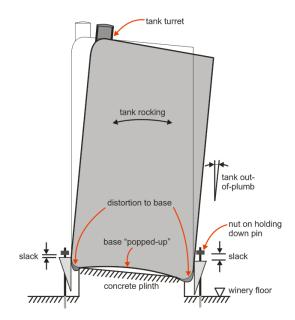
Figure 6: A characteristic damage state for plinth mounted tanks is tank settlement and "knuckle-squash" at the tank floor.
