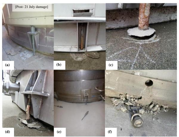
Anchorage failure by pullout, bolt tensile fracture and bolt shear failure
