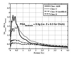
Figure 4: Average spectral shape curves for different soil classes when using rock motions.
