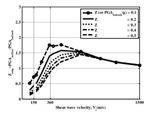
Figure 5: Relationship between normalised PGA and shear wave velocity for various Z factors when using rock motions.
