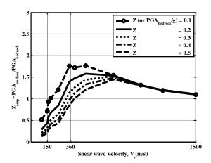
Figure 3: Relationship between normalised PGA and shear wave velocity for various Z factors (i.e. input motion intensity) when using rock motions.
