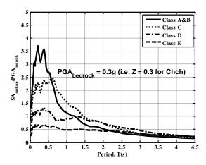
Figure 2: Average spectral shape curves for different soil classes when using rock motions.
