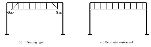
Figure 2: Common installation methods for suspended ceilings.
