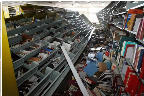
Figure 7: Typical damage to racks and shelves.
