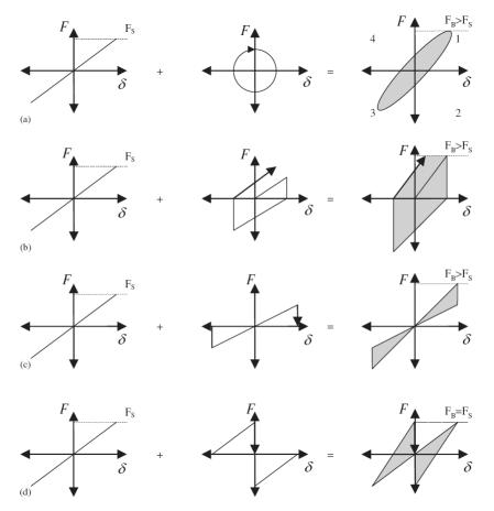
Figure 2. Schematic hysteresis for a) viscous damping; b) a 1-4 device; c) a 1-3 device; and d) a 2-4 device. Quadrants are labelled in the first panel, and  $F_B$  = total base shear,  $F_S$  = base shear for a linear, undamped structure.  $F_B$  >  $F_S$  indicates an increase due to the additional damping.
