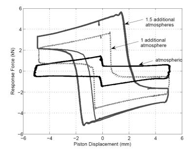
Figure 6. Comparison of devices working from atmospheric, 1.0 additional and 1.5 additional atmospheres of pressure.
