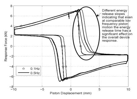
Figure 7. A large amount of air mass in the device leads to long energy release or reset times. The energy release time, indicated by a non-vertical line from peak force to the constant level, includes more of the overall motion with faster piston input motion, as illustrated here with piston motion of 0.1 and 0.5Hz.
