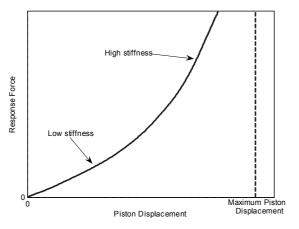
Figure 3. Force-displacement response of device showing low and high stiffness regions. The maximum piston displacement is indicated.
