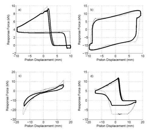
Figure 8. Device response to numerous control laws, some of which are one sided devices where one chamber is prepressurises while the other is held closed or works from atmospheric pressure. Experimental results are indicated with a solid line, while modelled results are shown with a dashed line.
