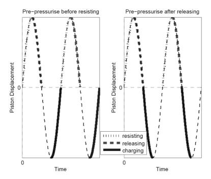
Figure 5. Configuration of charging the active chamber for pre-pressurising immediately prior to or following resisting motion.
