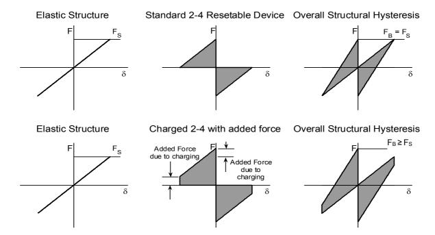
Figure 9. Schematic representation of resetable device contribution to overall structural hysteresis.  $F_B$  = total base shear, and  $F_S$  = base shear for a linear, undamped structure. Note that the addition of force from the charging of the device increases the overall base shear, whereas a standard 2-4 device does not.
