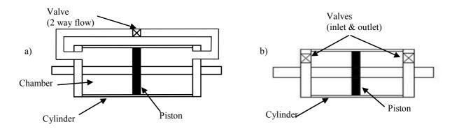
Figure 1. a) Original semi-active resetable device schematic as proposed by Jabbari and Bobrow [14]; b) Separated chamber design schematic with a valve controlling each chamber, thus removing interdependency of chamber.
