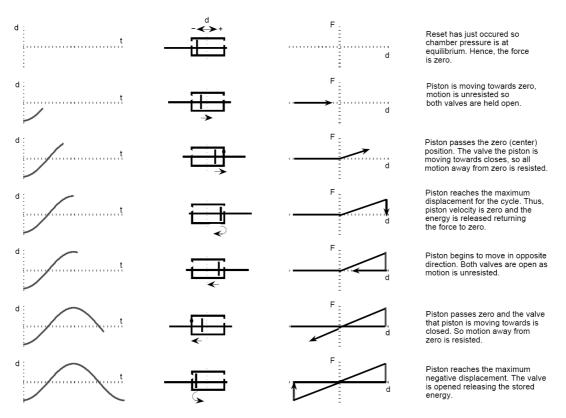
Figure A-2. Schematic showing one cycle of device under the 1-3 control law. The first column shows the piston displacement with respect to time. The second column shows a diagram of the device indicating the piston motion direction and the valve states. The third column shows the ideal force-displacement response.
