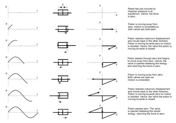
Figure A-3. Schematic showing one cycle of device under the 2-4 control law. The first column shows the piston displacement with respect to time. The second column shows a diagram of the device indicating the piston motion direction and the valve states. The third column shows the ideal force-displacement response.
