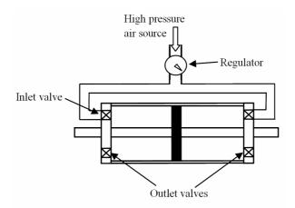
Figure 4. High pressure device schematic indicating inlet and outlet valves and high pressure air source.
