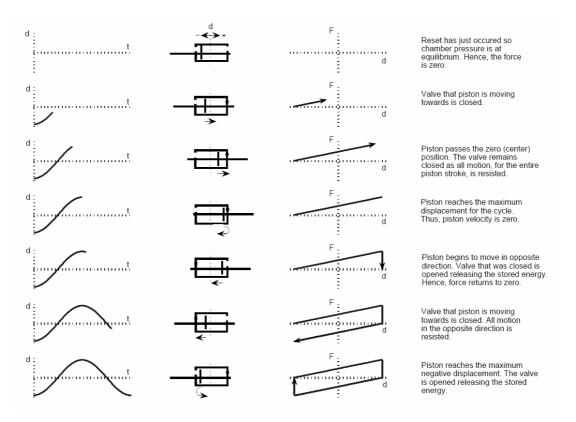
Figure A-1. Schematic showing one cycle of device under the 1-4 control law. The first column shows the piston displacement with respect to time. The second column shows a diagram of the device indicating the piston motion direction and the valve states. The third column shows the ideal force-displacement response.
