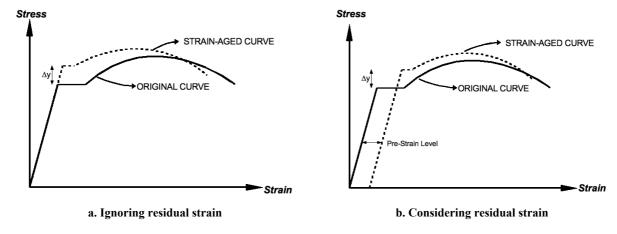
Figure 6: Comparison of stress strain curves of original and strain-aged bars.
