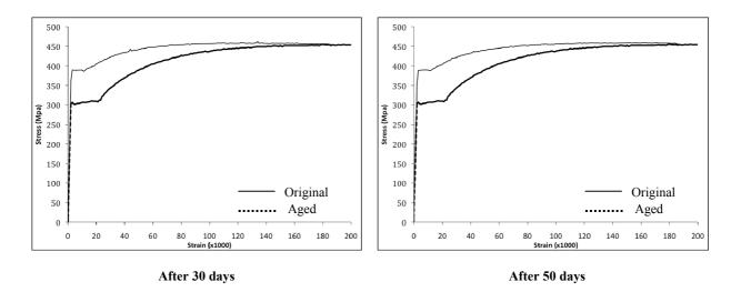
Figure 9: Average stress-strain curves of strain-aged samples tested with a pre-strain of 15 &
