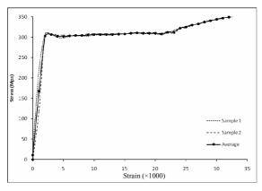
Figure 4: Stress-strain curves of the two benchmark specimens and the average stress-strain curve.
