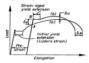
Figure 1: Schematic illustration of strain-ageing effect on stress-strain behaviour of reinforcing steel bars.
