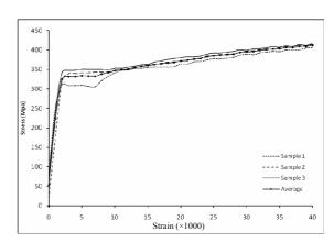
Figure 5: Individual and average stress-strain curves for specimens pre-strained to 10<sub>8</sub>, tested after 50 days.
