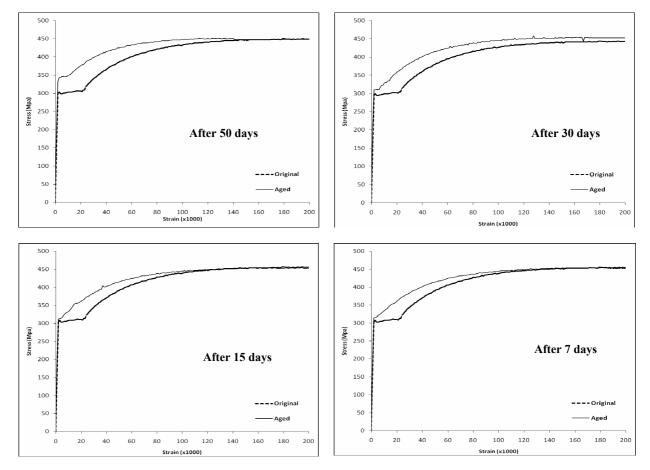
Figure 7: Average stress-strain curves of strain-aged samples tested with a pre-strain of  $10\varepsilon_{\rm p}$
