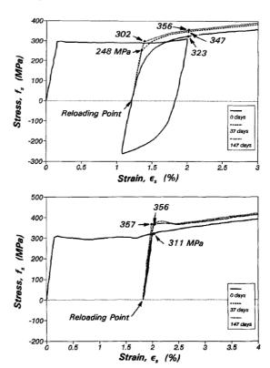
Figure 2: Cyclic and monotonic stress-strain behaviour (Posada 1992).
