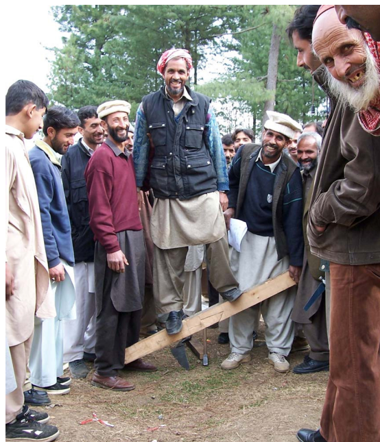
b) Testing strength of a timber joint (source: Kubilay Hicyilmaz).
