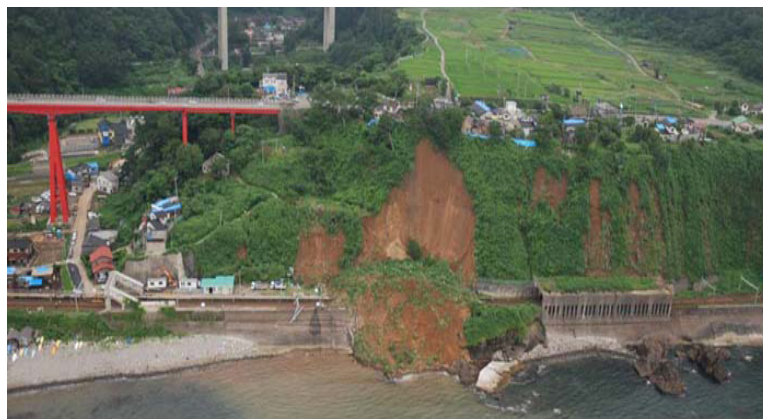
Figure 3: Slope failure near JR Omigawa station (photo by Kokusai Kogyo Co. Ltd).
