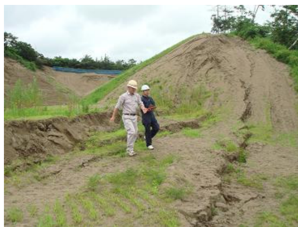
Figure 6: Top photo: liquefaction-induced collapse of the road leading to Kashiwazaki Incinerator Plant; Bottom photo: quarry site immediately to the right of the road.
