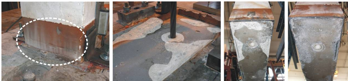
Figure 13. Damage state after removal of the precast wall from the foundation; Left: Dust flume on steel confining plate indicating expulsion of crushed concrete, Left Centre: Foundation recess with residual concrete, Right Centre: Rocking toe region (closest to mass), Right: Rocking toe region (furthest from mass).
