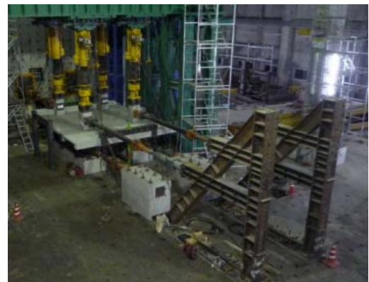
Figure 10: Loading set up at structural testing laboratory, Building Research Institute, Tsukuba.
