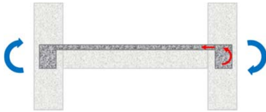
Figure 2: Beam component test with slab being anchored to transverse beams.
