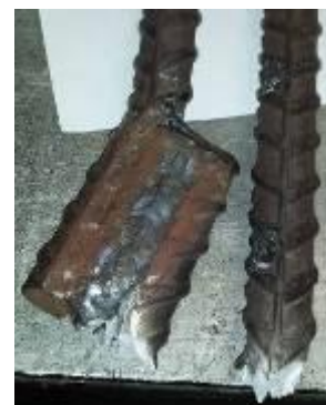
Figure 3: Fracture of double lap splice at weld.
