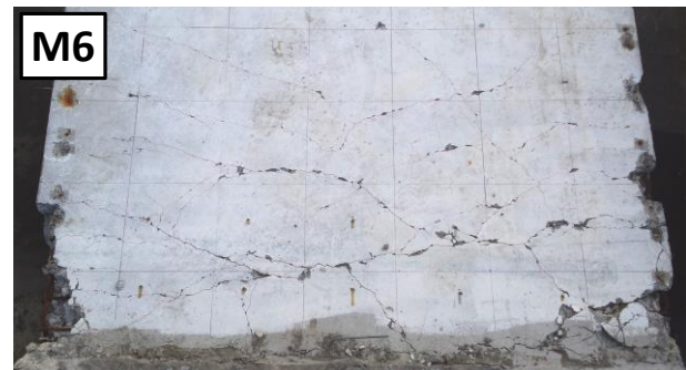
Figure 5: Damage of original specimens at the base of the wall after the completion of testing.
