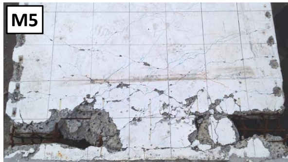
Figure 5: Damage of original specimens at the base of the wall after the completion of testing.
