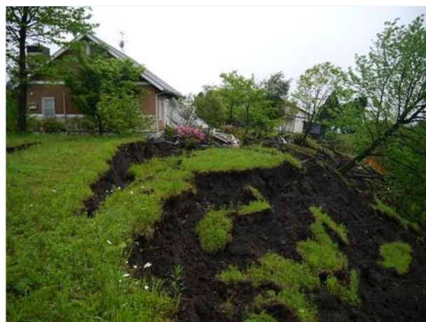
Photo 12: Toe area of the translational slide/slump at Tokyu Country Town showing the transition from sliding to slumping towards stream (N 32.8805; E 131.0025).
