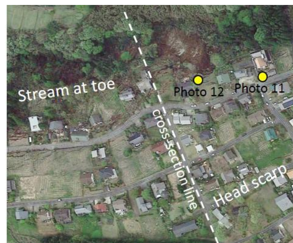
Figure 11: Google Earth image of the earth slide/slump at Tokyu Country Town (Location 12 in Figure 2). This landslide damaged about 40 homes.
