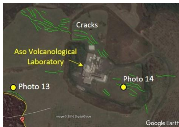
Figure 13: Google Earth image of the incipient landsliding at the Aso Volcanological Laboratory. Location 8 in Figure 2.
