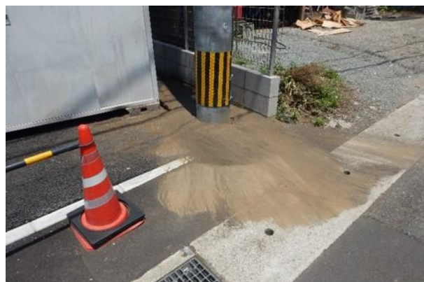
Photo 21: Traces of sand ejection adjacent to power pole in Kumamoto City (N 32.7583; E 130.6823).
