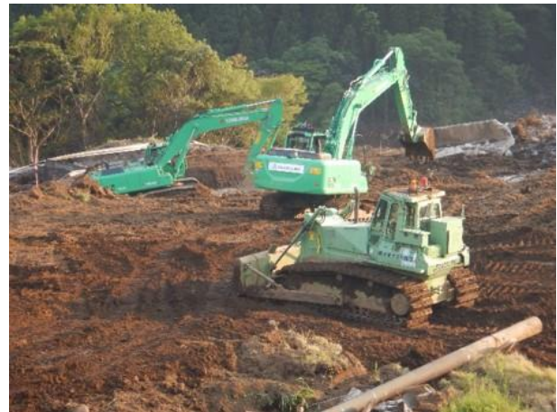
Photo 53: Remotely-controlled machines used to rescue buried construction equipment (N 32.8776; E 130.9764).
