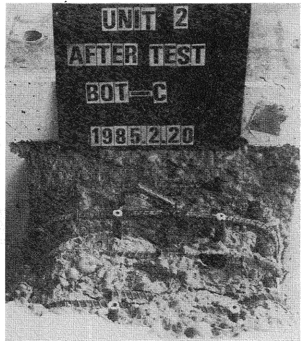
(b) Unit 2 at \mu_N = 12 . The 90° hooks at one end of the interior cross ties have opened.
